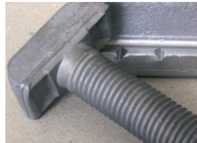
Notch teeth of the bolt press into the channel lips
